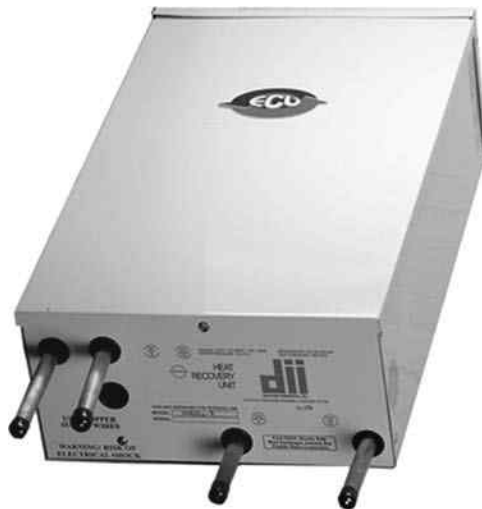
FIGURE 13-1 An ECU is used to recover heat from a direct-expansion air-conditioning system and channel that heat into a domestic hot-water tank, providing essentially free water heating and increasing the efficiency of the air conditioner. This is an example of load sharing. (ECU Energy Conservation Unit, Inc.) more appropriately called a desuperheater for domestic hot water generation.
