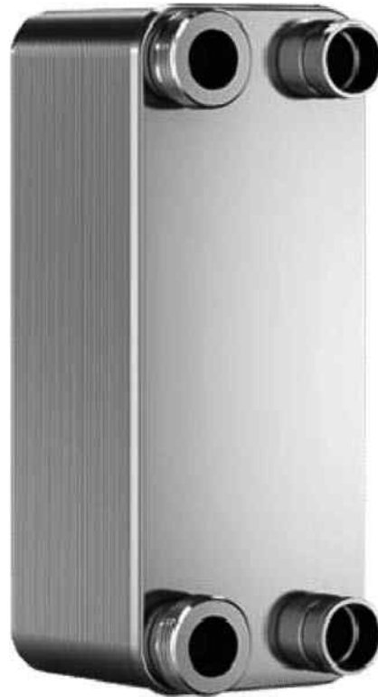
FIGURE 6-3 Typical brazed-plate heat exchanger. A small and very compact size for heat exchange is one of the definitive advantage for this type of heat exchanger. This type of heat exchanger can be quite efficient when designed properly. Antifreeze and inhibited solutions and pure water with little or no minerals are common requirements. This type of heat exchanger cannot be easily cleaned mechanically. (Water Energy Distributors.)
