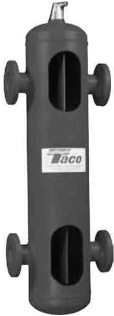
FIGURE 13-11 The hydraulic separator allows separate pumping of condenser water circuit to the heat-pump equipment and pumping of the fluid to the geothermal or ground-coupled portion of the system. This results in considerable pumping advantage and allows for load sharing. ( Taco, Inc. )
