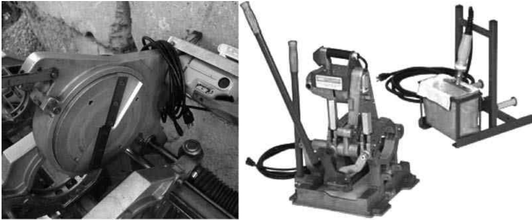
FIGURE 5-14 A mechanical facing tool prepares the ends to be joined by butt fusion.
