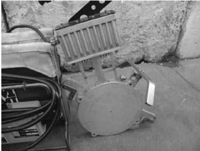
FIGURE 5-16 A fusion heating iron. The surface is coated with a nonstick Teflon material. Any oils or foreign debris will prevent a good fusion bond if present on the surface.
