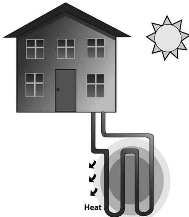
FIGURE 5-11 Thermal communication between boreholes can be a significant issue. In the illustration, the effect of rejected heat overlaps between the boreholes or the vertical piping, and compounding thermal saturation.
