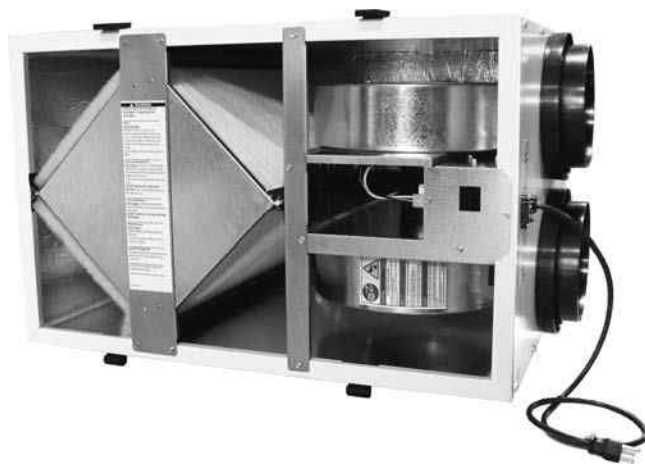
FIGURE 13-5 This exhaust-air ventilation recovery unit crosses the stream of conditioned air being exhausted from the building with outdoor air entering the dedicated outdoor air-conditioning unit. In this way, the air temperature and conditions entering the outdoor air unit are brought closer to the design air temperature for the building, saving considerable energy. (ERV, Inc.) Energy Recovery Ventilator
