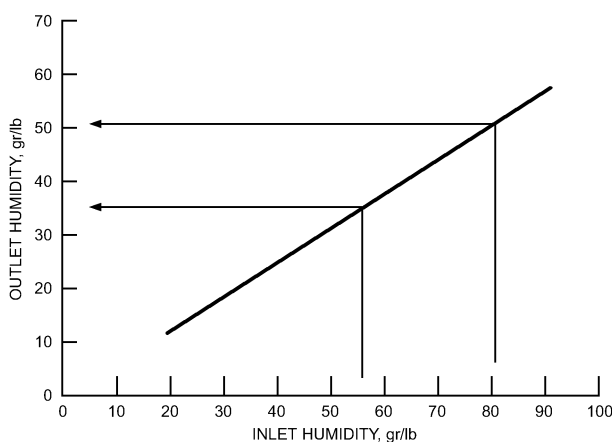
Fig. 9 Effect of Changes in Process Air Inlet Moisture on Dehumidifier Outlet Moisture
