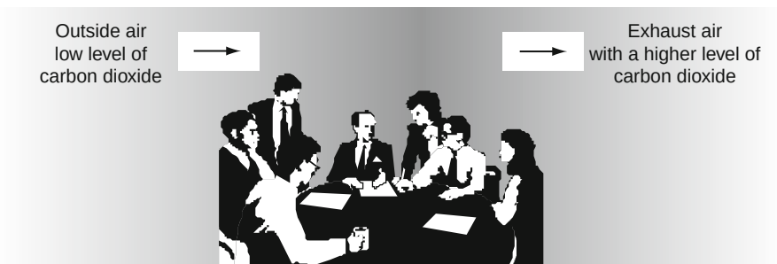
Figure 9-11 Ventilation Air Collecting \text{CO}_2 from Occupants
