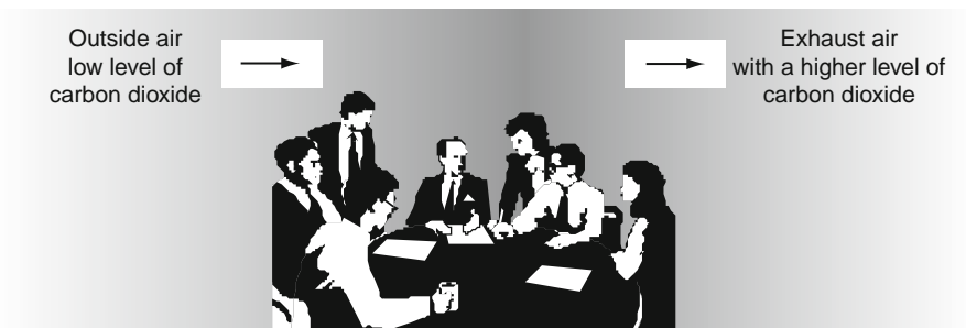
Figure 9-11 Ventilation Air Collecting \text{CO}_2 from Occupants
