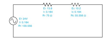
Figure 4–9 Circuit values for the series circuit are determined. (Source: Delmar/ Cengage Learning)
