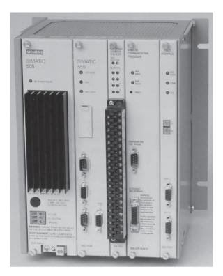
Figure 58-2 Plug connections located on the CPU. (Courtesy of Siemens Energy and Automation, Inc.).
