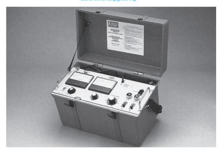
Figure 8-18 A dielectric test set. (Courtesy of Megger®)
