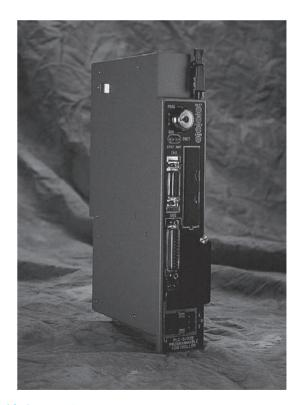
Figure 58-1 A central processing unit. (Courtesy of Allen-Bradley, a Rockwell International Company).
