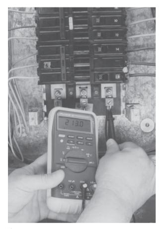
Figure 3–1 Voltmeter being used to test the voltage of a panel. (Source: Delmar/Cengage Learning)
