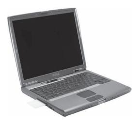
Figure 58-5 A notebook computer is often used as the programming terminal for a PLC. (Courtesy of Dell Computers).
