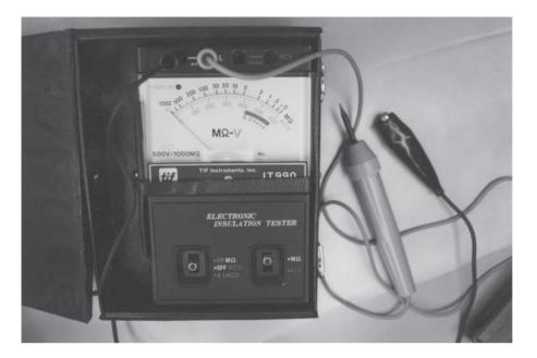
Figure 40-16 A megohmmeter for testing insulation resistance. (Source: Delmar/ Cengage Learning)
