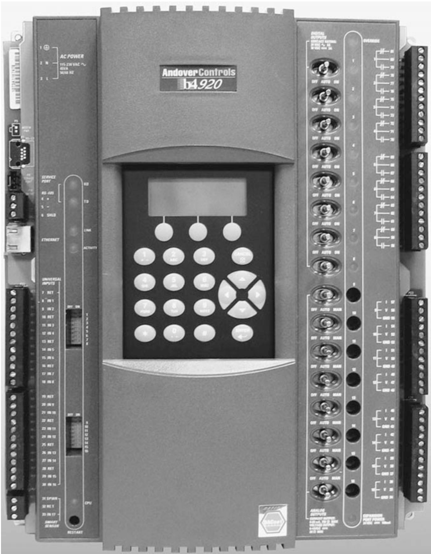
Fig. 5.65 A BACnet advanced application controller [5]
