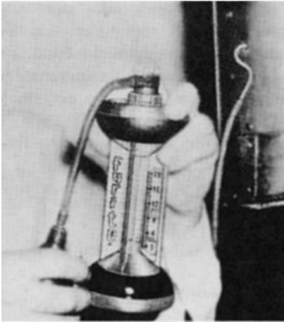
Figure I-43 Bacharach Fyrite CO 2 indicator.
