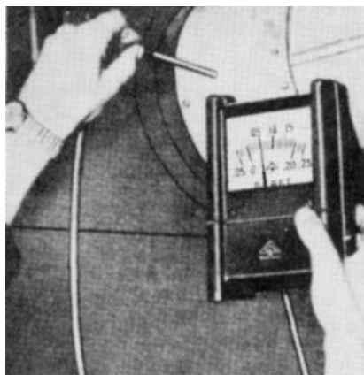
Figure I-45 Bacharach model MZF draft gauge.
