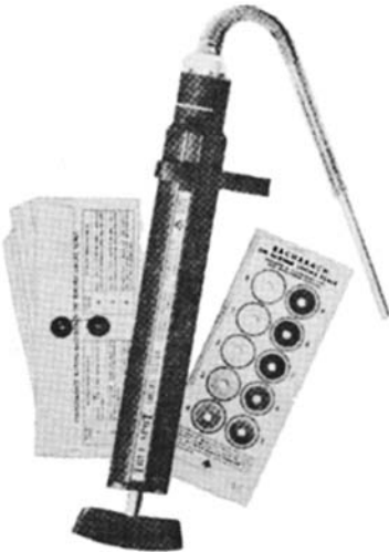
Figure I-40 Bacharach true-spot smoke tester.
