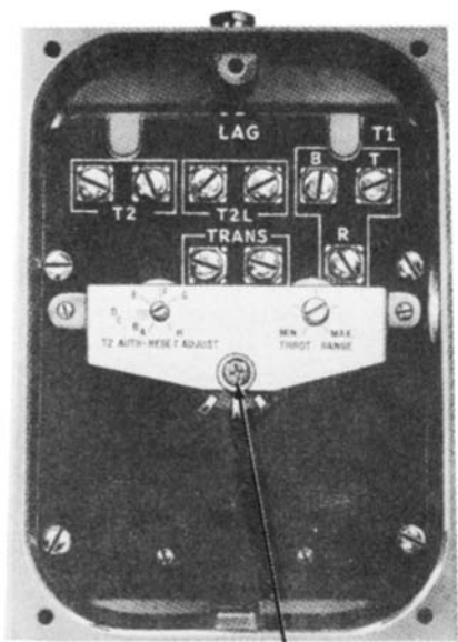
FACTORY CALIBRATION POTENTIOMETER DO NOT ADJUST
