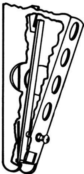
Figure 6-18 Flat-blade bimetal sensing element.
