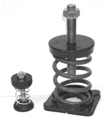
Figure 5-4 Two types of spring floor mounts. The mount on the left is for low loads and static deflections of less than 25 mm. The mount on the right is for larger loads and static deflections greater than 25 mm.
