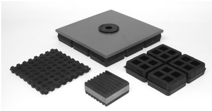
Figure 5-1 Elastomeric pads. The elastomeric bushing inserted in the metal load-distributing plate prevents metal-to-metal contact between the plate and its thru-bolt.
