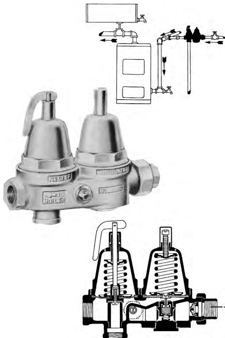
Figure 15-68 A combination relief/regulator valve (Type CBL).
