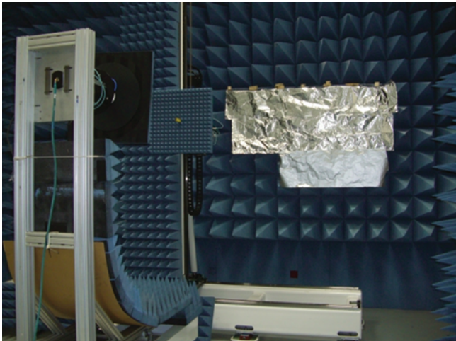
Figure 12.82 NSI-300V-12 × 12 system installed within a partially absorber lined chamber. Artificial scatterer introduced is also shown
