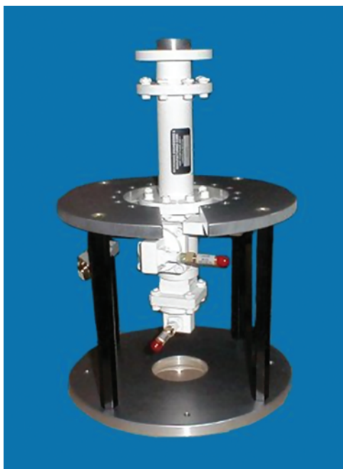
Figure 12.5 Picture showing back of choked circular waveguide probe showing OMT and dual coaxial ports
