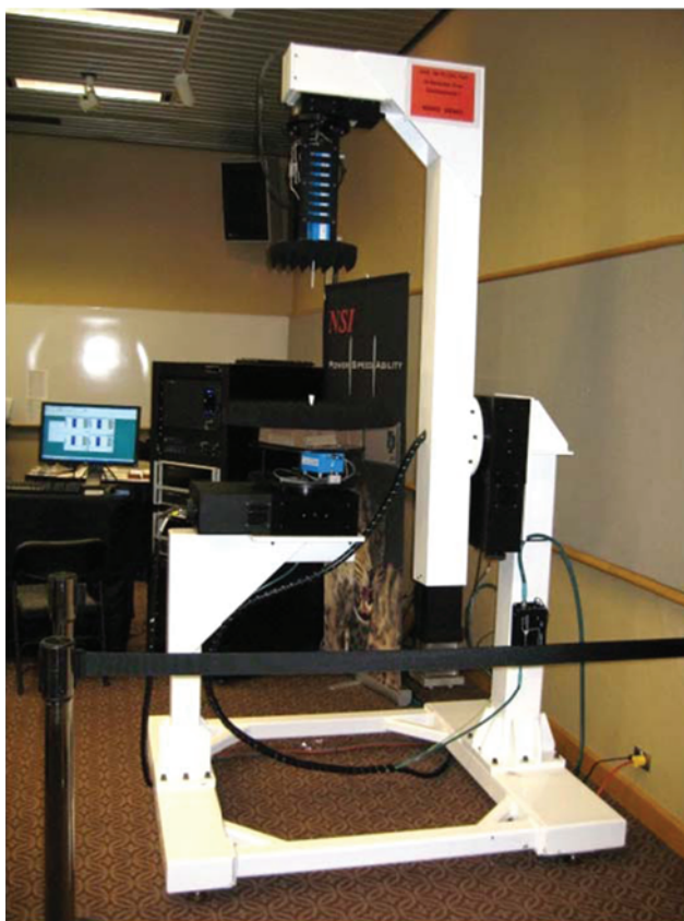
Figure 10.33 NSI swing-arm scanner shown with 75 GHz RF sub-system. Arm is parked in the \theta = 0^\circ location. Frequency up- and down-conversion units are mounted immediately behind the probe and AUT (Picture used with permission of NSI-MI Technologies LLC)
