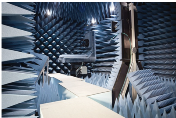
Figure 12.14 Far-field test system installed within an anechoic chamber (Picture courtesy of NSI-MI Technologies LLC)
