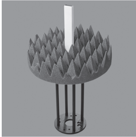
Figure 12.1 OEWG probe specifically designed for near-field measurements. Probes typically include absorber collar and chamfered aperture which are used to reduce the scattering cross-section of the probe
