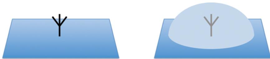
Figure 11.27 Wheeler Cap method for antenna efficiency measurement
