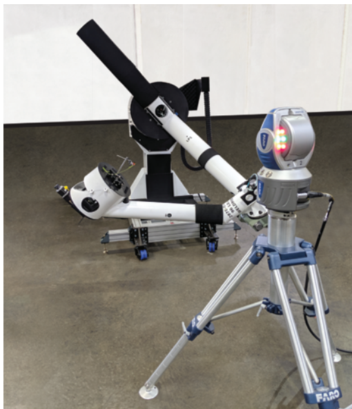
Figure 8.45 Structural measurement using a laser tracker. Note that only a portion of the full spherical surface can be evaluated
