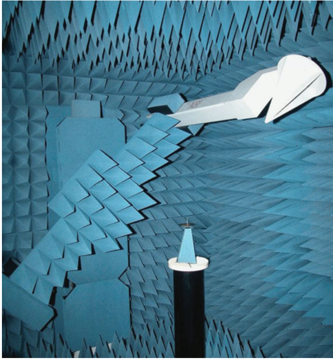
Figure 11.4 Overhead swing-arm spherical scanner. AUT is a monopole and the probe is a dual polarised, log-periodic 500 MHz to 18 GHz probe (Courtesy of NSI-MI Technologies LLC)
