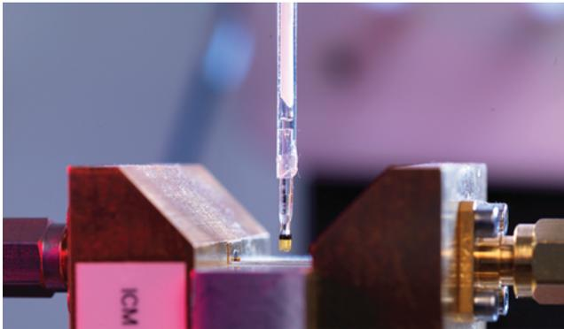
Figure 6.61 Close-up image of electro-optic probe scanning the very near-fields of a microwave device. The crystal probe can be seen in the centre of the image scanning immediately above the surface of the microwave transmission line. Pictured at the n3m-labs courtesy of NPL
