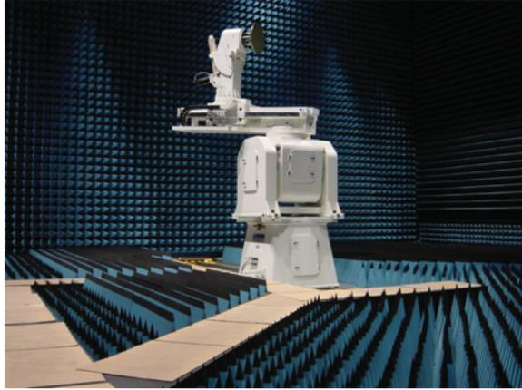
Figure 3.2 Seven-axis positioner (Courtesy of Leonardo MW)
