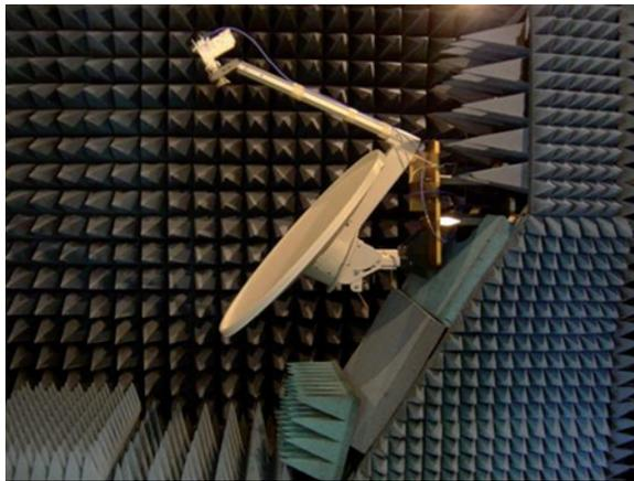
Figure 1.4 Offset parabolic reflector antenna
