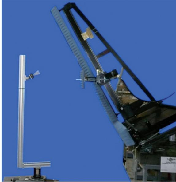
Figure 7.32 Conical near-field antenna measurements being acquired using an NSI-MI Technologies LLC combination planar-cylindrical positioning system
