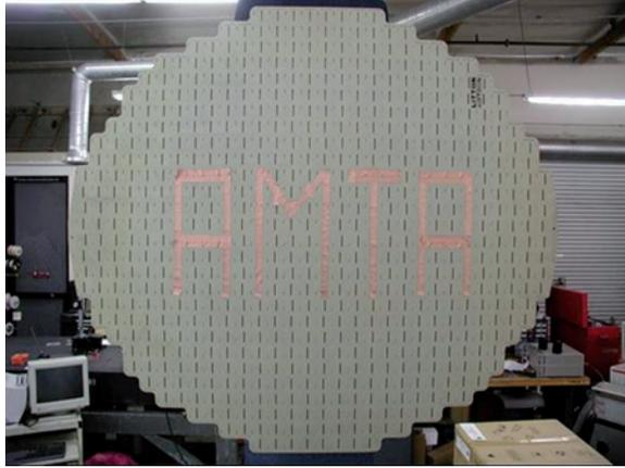
Figure 1.3 Slotted waveguide planar array antenna
