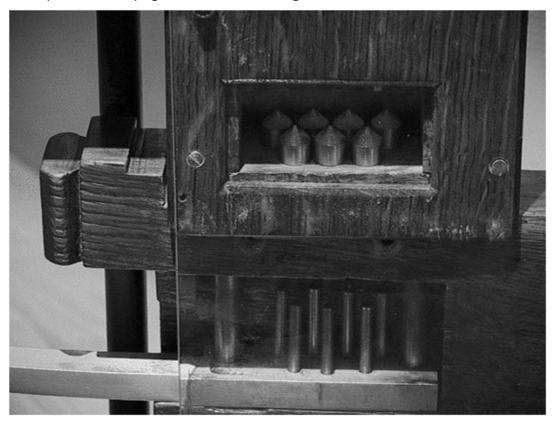
The original design of the pin tumbler lock was conceived more than four thousand years ago by the Egyptians. It was soon forgotten and lost in history until the mid-nineteenth century when Linus Yale decided it was time to produce a small, efficient, and secure lock. Yale's invention of the double-detainer locking theory in combination with a shear line offered an alternative to the lever tumbler, which was really the only mechanism that was both practical and secure at the time.
