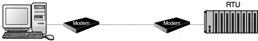
Figure 2.6 PC to RTU using a modem
