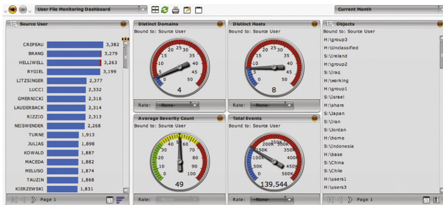
FIGURE 12.5 User activity related to file access as displayed by an SIEM.
