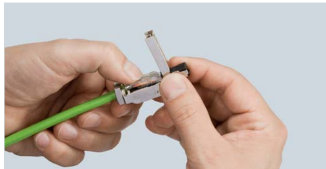
Insert the cores according to the color-coding as far as the end stop and press down on the contact lid
