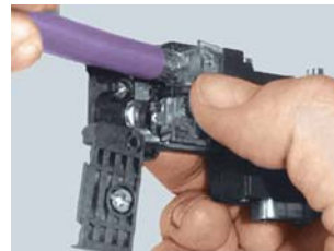
Stripping and assembly by means of insulation displacement
