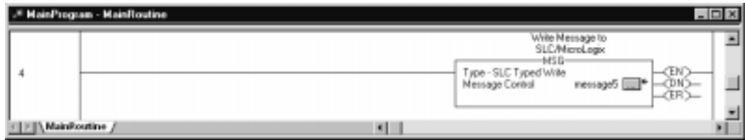
Figure 7.11 Example of a write MSG instruction from a Logix5550 to a SLC or MicroLogix controller
