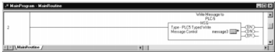
Figure 7.9 Example of a write MSG from a Logix5550 to a PLC-5 controller
