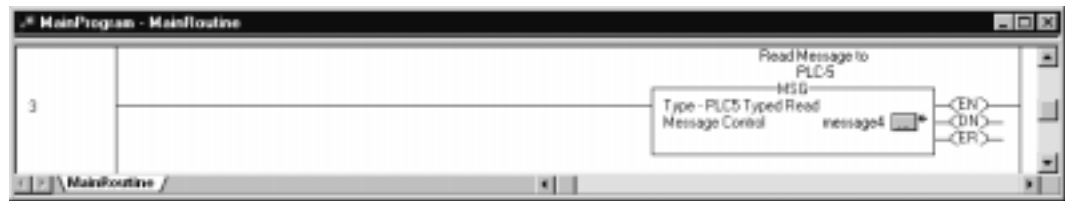
Figure 7.10 Example of a read MSG from a Logix5550 to a PLC-5 controller
