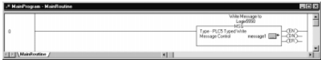
Figure 7.7 Example of a write MSG from a Logix5550 to a Logix5550 controller
