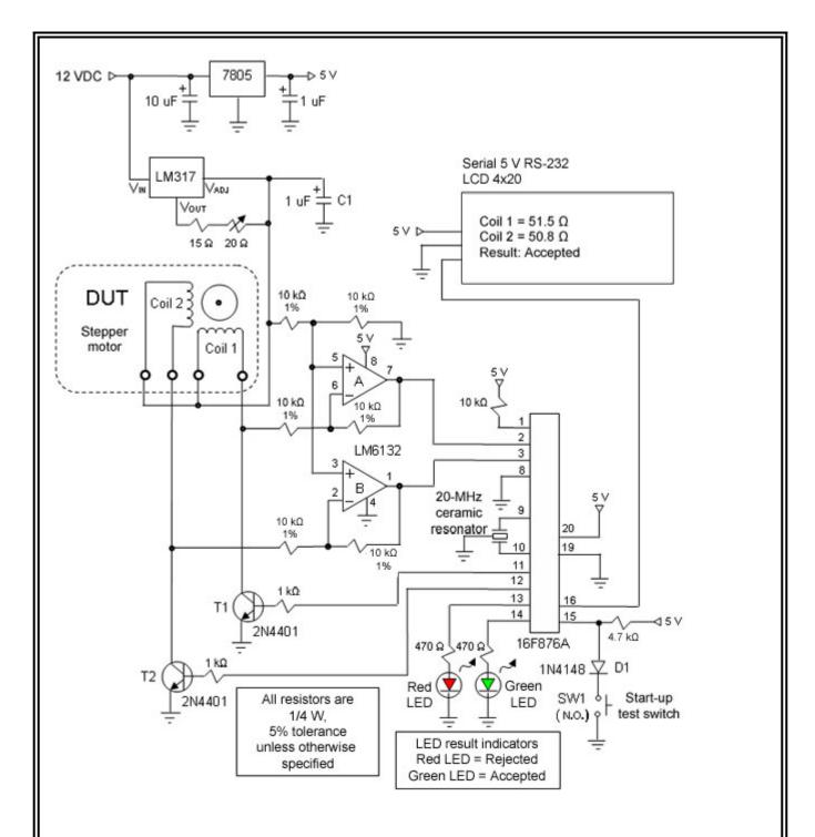
• Capacitor  $C_1$ , connected at the output of the constant-current source, will stabilize oscillations caused by the inductance of the winding coils from the stepper motor.
