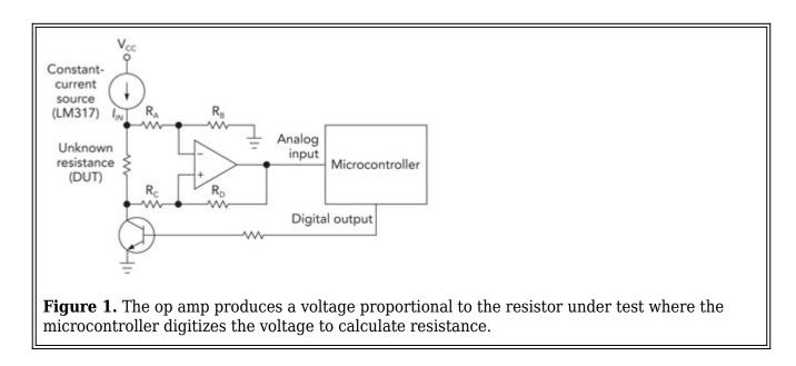
Next, define the scale measurement or digital value within the microcontroller. The nominal value of the DUT (device under test) should be close to half of the scale selected. Thus, you should set the full-range scale from 0  $\Omega$  to 100  $\Omega$ .
