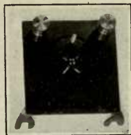
FIG. 111.—Mounted thermocouple with protecting cap removed
