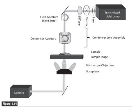
Layout of transmitted bright field microscope setup.
