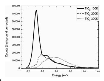
Temperature-dependent PL spectra of titanium dioxide films grown by atomic layer deposition on a silicon substrate. Note that lower temperatures tend to increase PL signal and to sharpen PL peaks. The largest peak (in this case around 3.3 eV) is usually the band to band transition and the smaller peaks at lower energies (like the small peaks at 1.7 eV) are defect states. The peak center is usually reported as the energy of the bandgap. Samples courtesy of Malcolm Hathaway.
