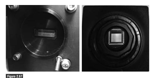
Camera chips come in different shapes. Long narrow formats are used for spectroscopic applications. Square formats are used for imaging applications.
