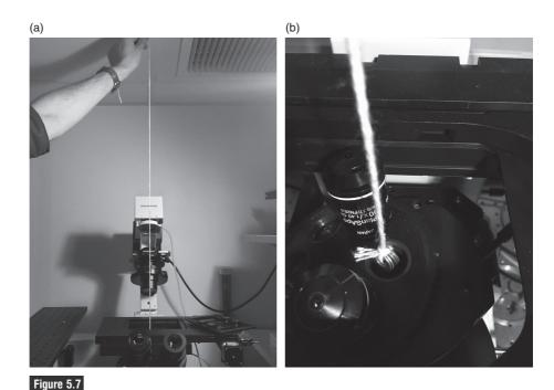
Plumb line being used to find true vertical from an empty microscope objective port.
