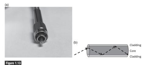
(a) End of a fiber optic cable. The glass fiber is in the very center of the tip. There is a polymer cladding around the glass fiber and then a metal jacket to help protect the fiber from being accidentally broken. (b) The cladding must have an index of refraction lower than the core for total internal reflection to occur at the interface.
