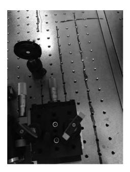
Drawing the beam path directly on the optics helps everyone remember the optical layout and where the laser beam is going. Laying out the optical path to go along the line of screw holes in the optics table helps make sure that the beam in your setup is going in a straight line.
