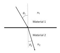
Snell's law describes how the direction of propagation of light will change when it encounters a material with a different index of refraction.
