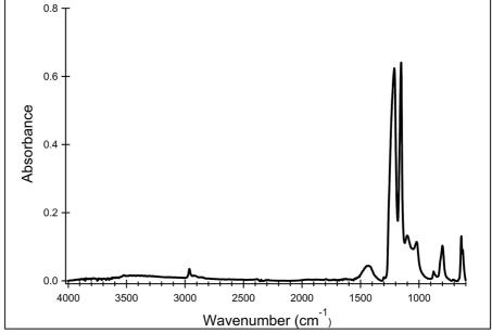
Transmission FTIR spectrum. FTIR spectra are sometimes plotted with percentage transmission (%T) on the *y*-axis and sometimes with absorbance units (Abs) on the *y*-axis.
