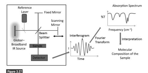
Schematic of Michelson interferometer inside a typical FTIR.
