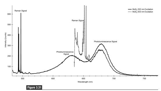
Raman and PL signals of  $MoS_2$  sample excited with 532 and 633 nm light. Raman peaks are shifted from the excitation line. PL peaks are always in the same spectral position and tend to be much wider. Sample courtesy of Luis Jauregui.
