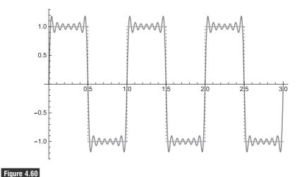
A seven sine wave fit to the one-dimensional image in Figure 4.57.
