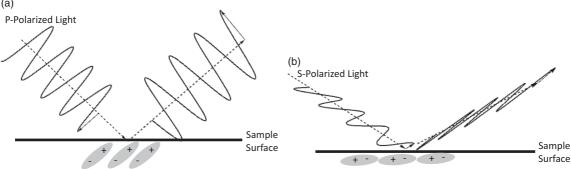
Dipole moments excited out of the plane of the sample surface
