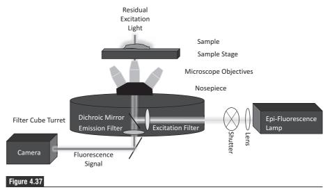
Lavout of an epi-fluorescence microscope.
