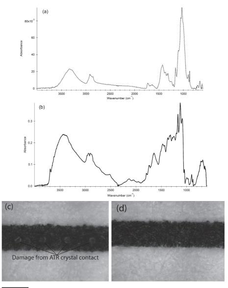
(a) ATR-FTIR spectrum; (b) specular reflection FTIR of the same sample; (c) damage of the sample due to contact with the ATR crystal; (d) sample undamaged by specular reflection FTIR. Sample courtesy of Elena Bulat.
