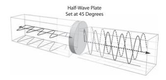
A half-wave plate (HWP or  $\lambda/2$ ) can rotate the polarization of linearly polarized light without changing the intensity of the beam. The exact orientation of the electric field in the output beam depends on the orientation of the fast axis of the half-wave plate with respect to the electric field in the input beam.
