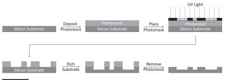
A basic photolithography process. First, a silicon substrate is coated with a thin film of photoresist. Then, the glass contact mask is placed on the wafer. The mask and wafer are exposed to UV light, and the mask is removed. Next, the wafer is developed in solvent meant to remove the exposed areas of photoresist. Next, a process is performed on the Si wafer, which only affects the wafer in the areas exposed by the openings in the photoresist. Finally, the photoresist is stripped away.
