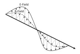
Light is electromagnetic radiation that consists of perpendicular electric and magnetic fields that are orthogonal to the direction of the propagation of light. The electric field is traditionally denoted with E and the magnetic field is traditionally denoted with B. The magnetic field is largely ignored in optics and only the interaction of the electric field with matter is considered.
