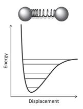
Vibrational energy level diagram showing a Morse potential energy well. Displacement is the distance between the atoms. As the atoms get too close, they start to repel each other, making the potential energy barrier rise sharply. As the atoms are stretched too far apart, the bond will eventually break. In FTIR, the molecule moves up a vibrational energy level by absorbing an infrared photon that has the exact same energy as the difference between the initial and the final energy levels.
