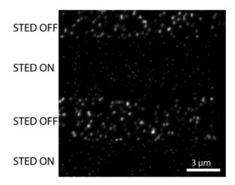
Demonstration of the improved spatial resolution of stimulated emission depletion microscopy. The sample was yellow/green 40 nm fluorescent beads imaged with 490 nm excitation and 590 nm STED lasers. The STED laser was turned on and off to show the enhanced spatial resolution. Image is courtesy of Dr. Douglas Richardson.
