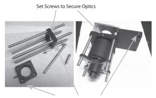
Set Screws to Allow Frame Motion Along the Posts
