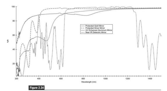
Reflectivity versus wavelength plots of three common mirror materials: silver, gold, and a broadband dielectric stack mirror designed for the near infrared region.
