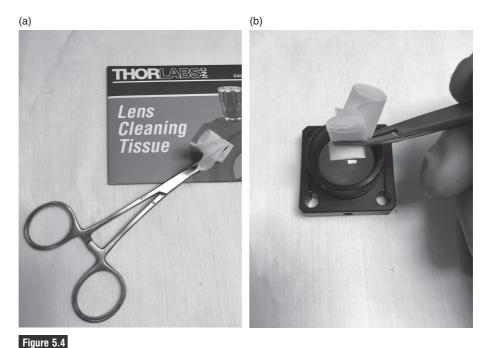
Cleaning optics using lens cleaning tissue. (a) Using forceps to secure a piece of lens cleaning tissue. (b) Cleaning the lens.
