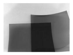
Two partially overlaid sheet polarizers. When the orientations of the polarizers are 90 degrees relative to each other, they are said to be crossed. Crossed polarizers will block all light as seen in the dark overlapping region in the middle. The single polarizer looks gray as it is blocking light of a specific polarization (about half the light in a typical unpolarized beam).
