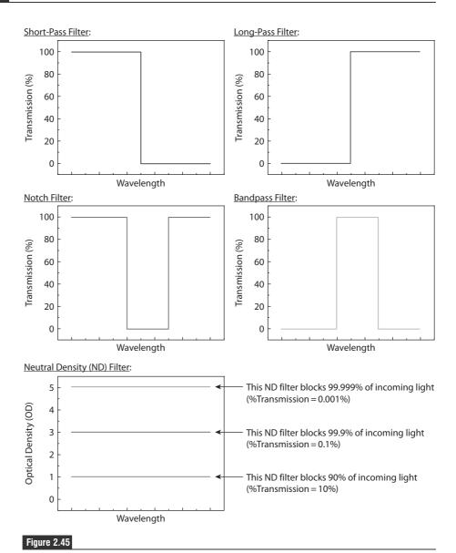
Typical transmission vs. wavelength characteristics of short-pass, long-pass, notch, bandpass, and neutral density (ND) filters.
