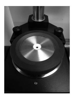
A single-bounce germanium ATR crystal with Teflon trough for liquid samples. A drop of liquid is placed on the Ge crystal and then the ATR-FTIR spectrum can be collected. The trough would also be used for powdered samples in conjunction with a pressure arm to press down on the powder and make sure there is good contact between the crystal and the powder. The trough can be removed for larger solid samples.
