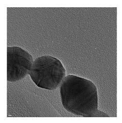
TEM image of gold nanoparticles suspended on a carbon film. Lattice fringes corresponding to columns of atoms in the gold particles are clearly visible. Scale bar, 2 nm.
