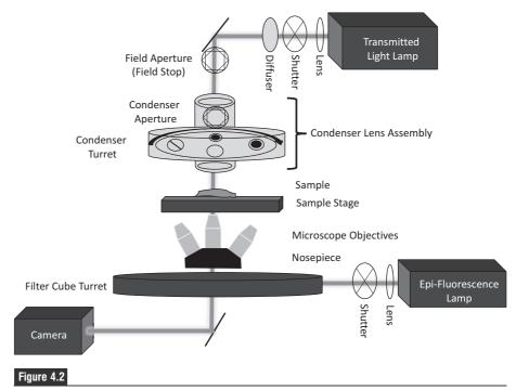
Schematic of an optical microscope. Even in a simplified cartoon form, a microscope has many parts to understand. A good practice is to follow the light path to understand what is going on.
