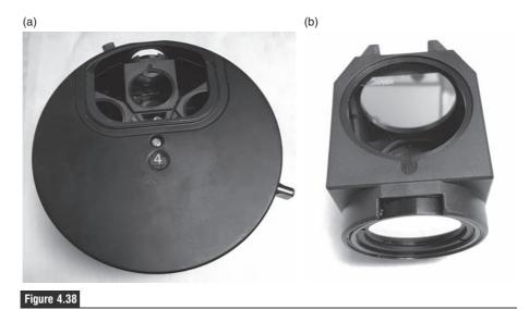
(a) Fluorescence filter turret. (b) Fluorescence filter cube.
