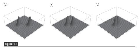
(a) Two fully resolved points. (b) Two overlapping but resolvable points. (c) Two unresolvable points.
