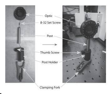
Assembled optical mount using a clamping fork base. A washer is used between the screw and the clamping fork for extra stability. In this case, the post holder has a flange at its base, allowing the clamping fork to clamp it into position. Note that use of a clamping fork allows the optic to be positioned anywhere within a certain distance (determined by the length of the clamping fork) of the screw.
