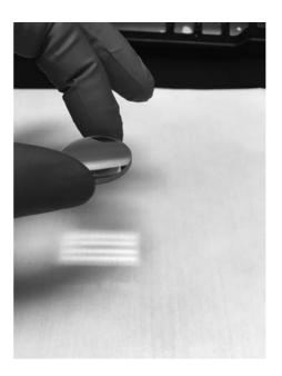
The focal length of an unmarked lens can quickly be determined by focusing the image of the ceiling light fixture. The distance between the lens and the image is the focal distance of the lens. Wearing gloves when handling unmounted optics prevents fingerprints on the optics.
