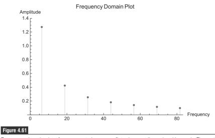
Frequency domain plot of component sine waves fit to the one-dimensional image in Figure 4.57.
