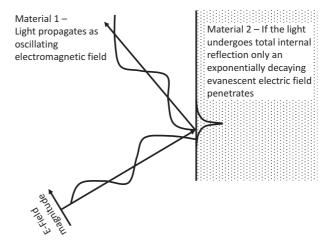
When light undergoes total internal reflection, all the light is reflected back from the interface and only an exponentially decaying evanescent electric field penetrates into material 2. The penetration depth depends on the wavelength of light and the indices of refraction of the two materials but it is typically several hundred nanometers.
