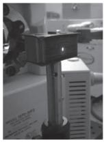
Beam blocks. An unmounted beam block is shown on the left. Right, a beam block blocking a 405 nm laser.
