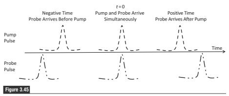
The time resolution of the measurements is determined by the relative time of the pump and probe pulse arrivals at the sample. Negative times correspond to the probe arriving before the pump. Time zero corresponds to the instant when the two pulses arrive simultaneously. Positive time corresponds to the probe arriving after the pump.
