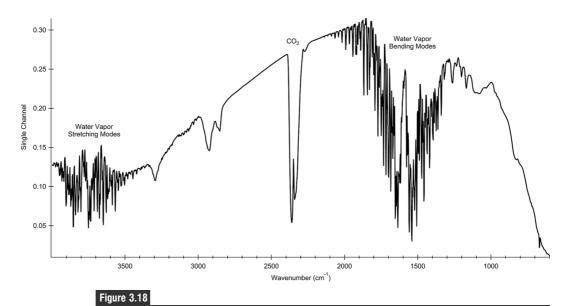
Background measurement showing the blackbody radiation shape to the intensities of the light as a function of wavelength and absorbances from atmospheric water vapor, carbon dioxide, and some coatings on the optics.
