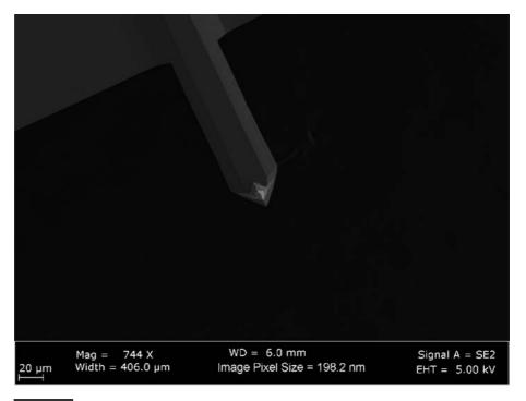
Scanning electron microscopy image of an AFM tip. The cantilever sticks out from a chip in the top left of the image. The low-contrast pyramid at the end of the cantilever is the actual AFM tip (pointing up toward the viewer in this image) that interacts with the sample.
