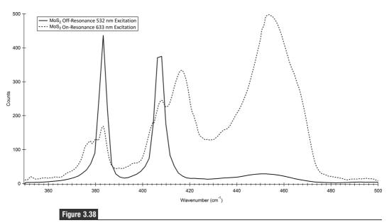
Resonance Raman (633 nm excitation) and off-resonance Raman (532 nm excitation) of MoS<sub>2</sub>. The peaks that were too weak to see with the off-resonance 532 nm excitation are enhanced with the 633 nm resonance Raman excitation.
