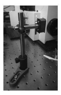
A right-angle post clamp used to mount a beam block perpendicularly to the axis of another post.
