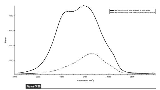
Polarized Raman measurements of water.
