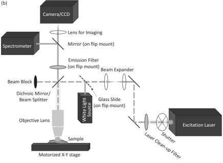
Schematics for the various configurations of PL imaging and spectroscopy. Dotted lines correspond to excitation light, whereas solid lines correspond to emitted light from a sample (or a plasma line from the laser). The gray rays correspond to broadband white light.
