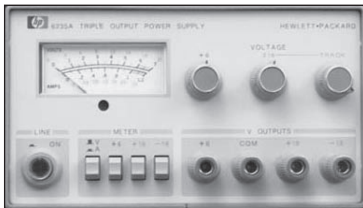
Figure 7.22 Example of a full-featured instrumentation power supply.
