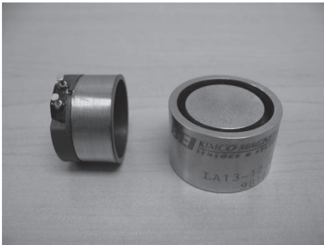
Figure 10.4 Photograph of a voice coil iron core and coil.
