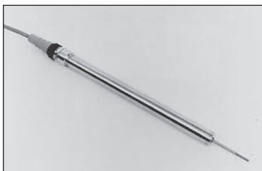
Figure 9.11 Commercial LVDT. (Courtesy of Sensotec, Columbus, OH)
