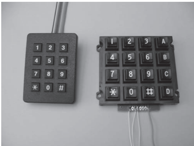
Figure 7.10 Photograph of 12-key and 16-key numeric keypads.
