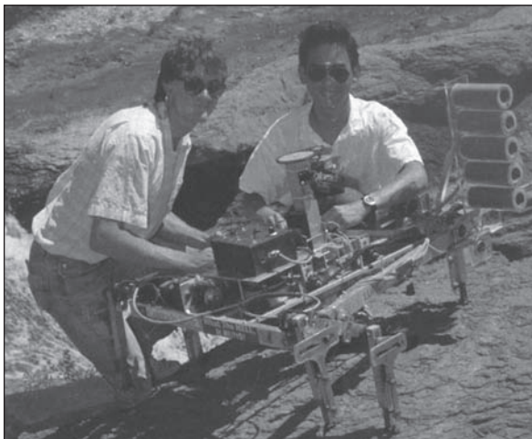
(a) "Lurch"—Scotch yoke mechanism leg design (1989)
