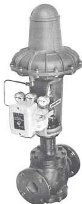
Fig. 10-2. Type C: Vernier Valvactor positioner provides fast, precise valve positioning proportional to 20 to 100 kPa or 3 to 15 psi.
