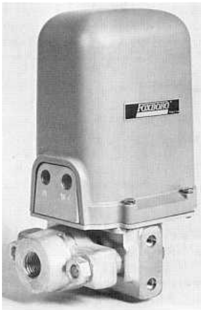
Fig. 2-24. Model 11GM pressure transmitter is a force-balance instrument that measures pressure and transmits it as a proportional 3 to 15 psi or 20 to 100 kPa pneumatic signal.
