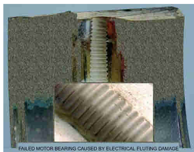
Fig. 8 Fluted Bearing from VFD-Induced Electrical Bearing Current Discharges (Oh and Willwerth 2008)
