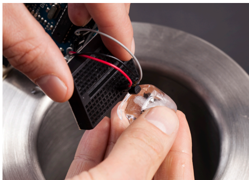
Figure 3-19. Testing the LM35 with an ice cube
