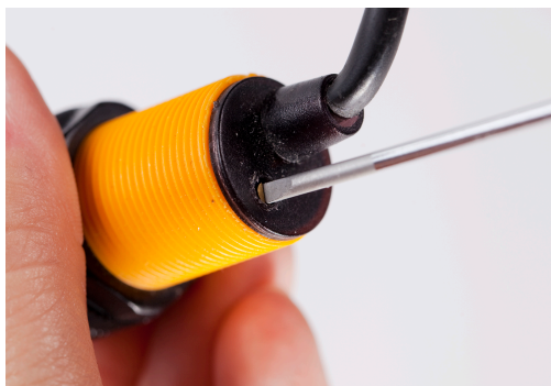
Figure 3-8. Adjusting the infrared sensor
