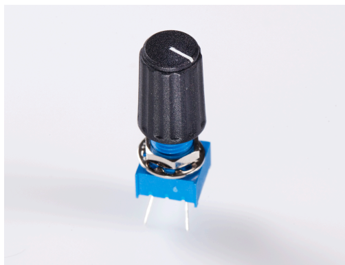
Figure 3-10. Potentiometers can measure rotation
