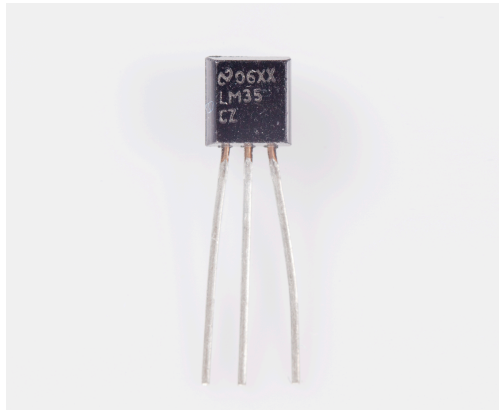
Figure 3-17. LM35 temperature sensor
