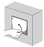
2) Peel the release paper off the back of the new protective sheet. Position the hole for the USB environmental protection cover of the sheet to the USB environmental protection cover of the GOT. If the protective sheet without the hole for the USB environmental p cover is attached, position the sheet from the upper left of the GOT. of the prote
