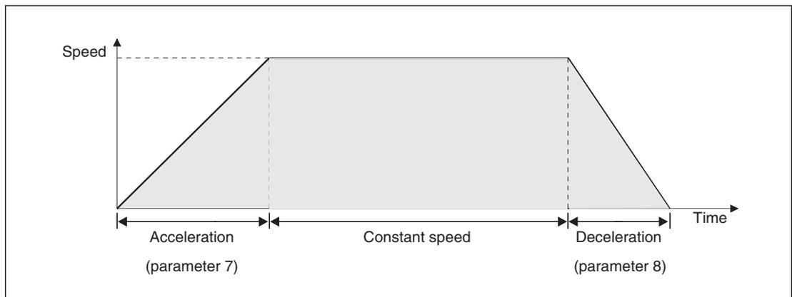
In this example we are going to use an FR-D700 series inverter to power and control the belt using the speed/time pattern shown in the graph above. The configuration is as follows:
