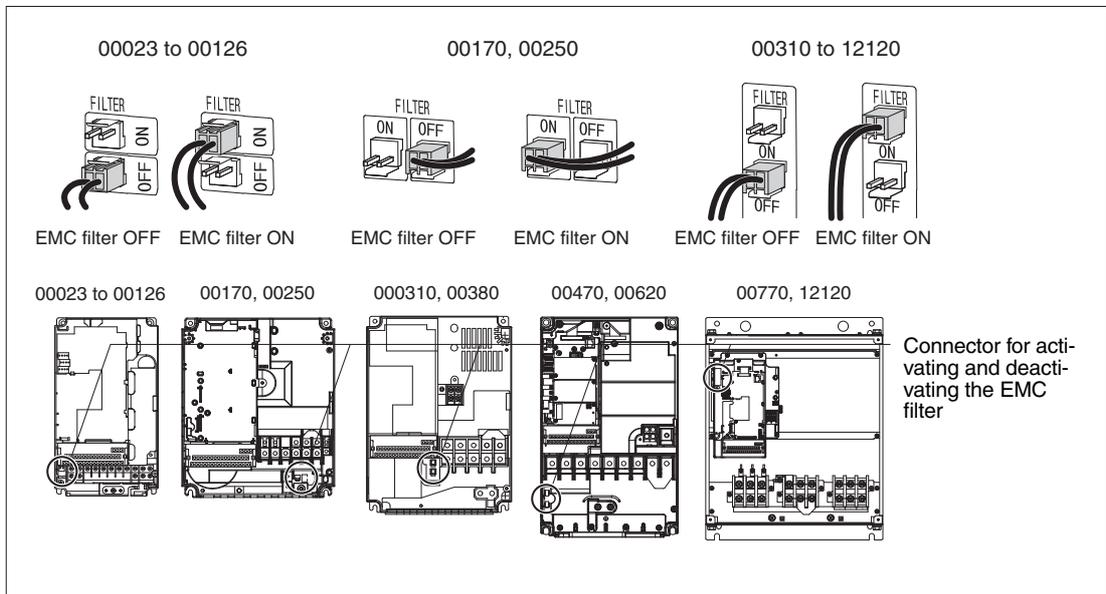
The connector must always be installed, either in the ON position or in the OFF position.
