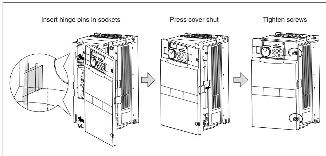
**Removing and replacing on models from FR-F740-00770/FR-A740-00770**
