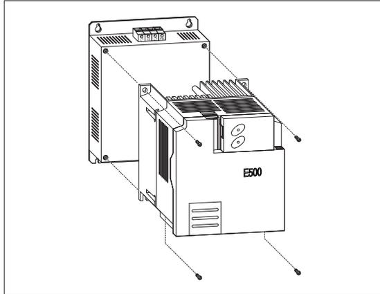
The EMC filters of the FR-D700 and FR-E700 series are installed beside or behind the inverter, depending on their design. Installing the filter behind the inverter has the advantage that the filter does not take up any additional space in the switchgear cabinet.
