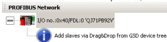
Slaves are added by dragging a slave type from the GSD tree and dropping it in the project tree. The configuration settings of master and slaves are accessed via entries in the context menu.
