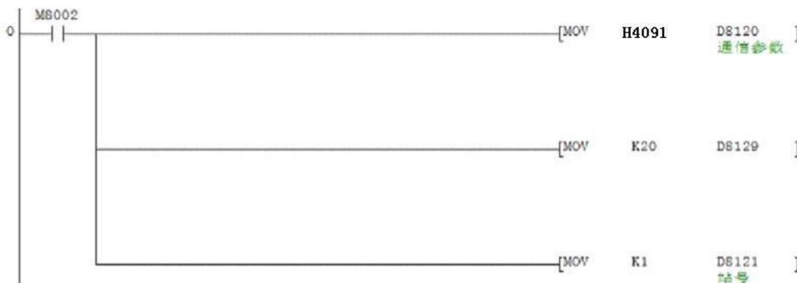
example:Set PLC as MODBUS RTU slave, station number 1,19200,8,N,1
