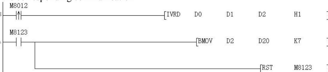
D0 for reading the station number (high 8) and the command code (low 8), such as the value of H103 D0, is the number of stations
