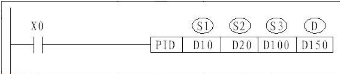
This directive is used to carry out PID control of the PID computing program.
