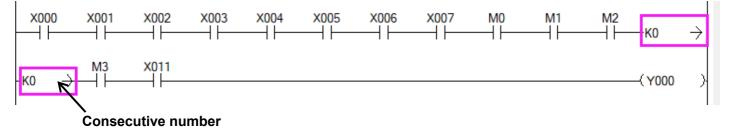
The operation of the ladder program is scanning from the upper left to the lower right. The coil and application instruction operation box belong to the output processing, and are placed at the far right in the ladder diagram.
